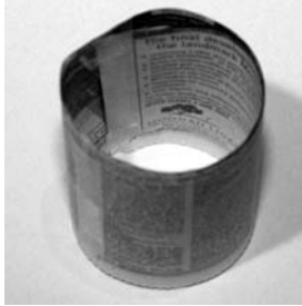
Figure 4.13(b) Cylindrical collar crushing specimen
