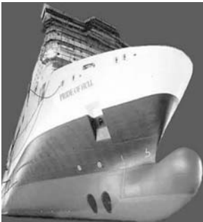
Figure 8.29 Bulbous bow on vessels in dry dock and at sea
