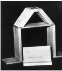
(c) Structure mass 87.7 gm failed at 522 N
