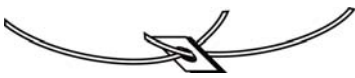
Figure 3.19(a) Schematic sketch of one type of friction joints used in the balsa “string suspension bridge”
